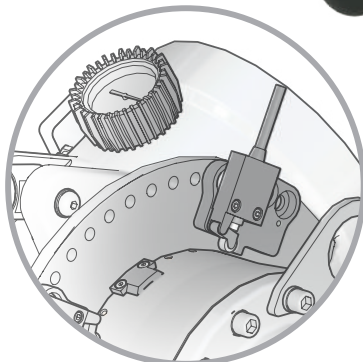
Vertical and horizontal electric stops
